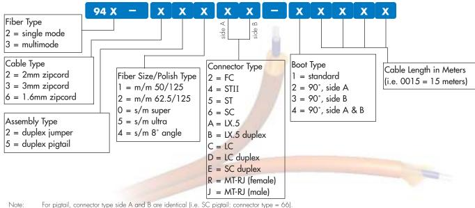
For pigtail, connector type side A and B are identical (i.e. SC pigtail: connector type = 66). For hybrid jumpers, use the lowest number first (i.e. SC to FC: connector type = 26). LX.5, LC and MT-RJ jumpers not available for 3mm jacketed cable. 90° boots are not available with 900µm fiber and certain connectors.
