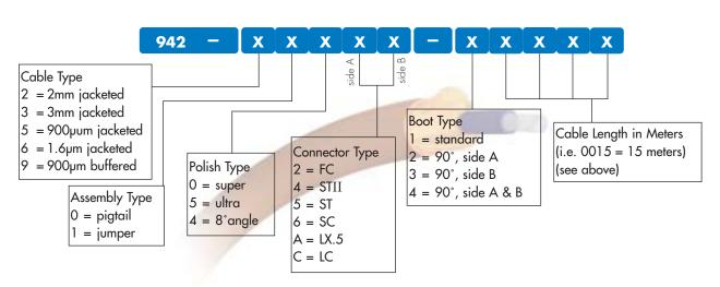
Note: For pigtails, connector type side A and side B are identical (i.e. SC pigtail: connector type = 66). For hybrid jumpers, use the lowest number first (i.e. SC to FC: connector type = 26).
