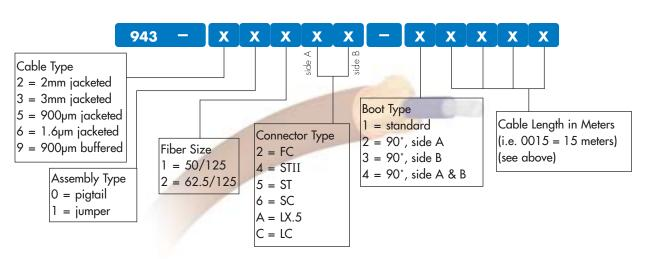
Note: For pigtail, connector type side A and B are identical (i.e. SC pigtail: connector type = 66). For hybrid jumpers, use the lowest number first (i.e. SC to FC: connector type = 26). IX.5 and IC jumpers not available for 3mm jacketed cable.
